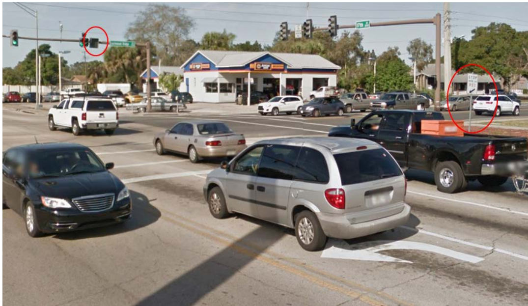
Figure 28 - Example 1 with both “NO TURN ON RED” and “STOP HERE ON RED” signs
