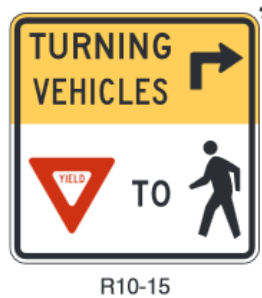
Figure 3 - “TURNING VEHICLES YIELD TO PEDESTRIANS” sign
