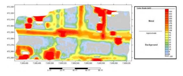
Figure 6. Screen capture. 2D plan map from TDEMI data collection – (these maps are often referred to as a heat map where red indicates metallic objects on the surface or in the subsurface). Courtesy of Cardno.
