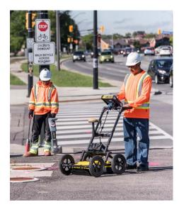
Figure 2. Example GPR SUE instrumentation (Sensors and Software LMX200<sup>™</sup> GPR) – photo courtesy of Sensors and Software.
