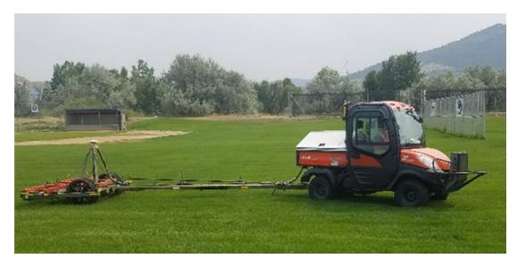
Figure 5. Photo of TDEMI towed array during R01B project work. Note this is a diesel-powered tow vehicle. Courtesy of Utility Mapping Service, Inc.
