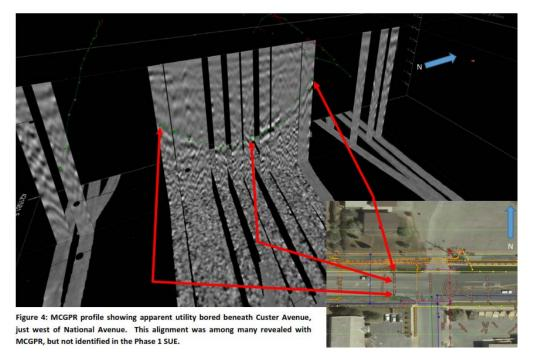
Figure 9. Screen capture. 3D imagery from MCGPR volumetric data set. Courtesy of Utility Mapping Services, Inc
