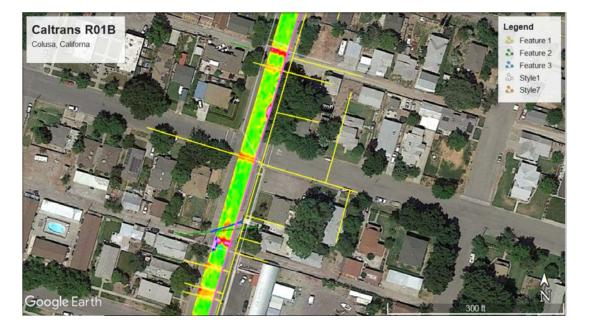
Figure 7. Screen capture. Draft 2D plan map (overlain on Google Earth Imagery) from TDEMI data collection – (known metallic utilities shown as thin yellow lines for comparison). Courtesy of Caltrans.
