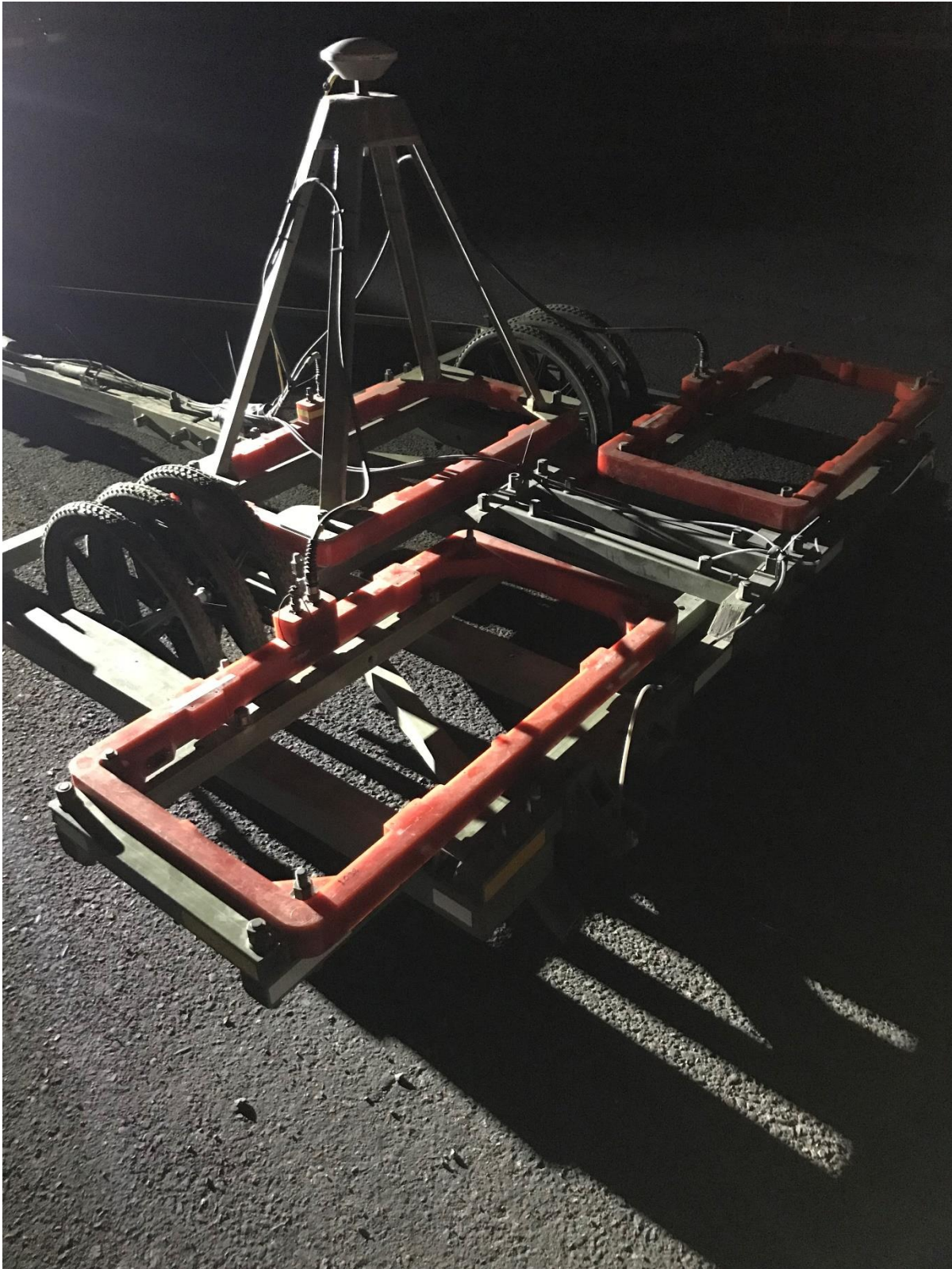
Time Domain Electromagnetic Induction (TDEMI) instrumentation used during the SHRP2 R01B Utility Locating Technology program for the MDT Custer Avenue project. Shown here is a towed-array of three Geonics EM61-MK2A geophysical instruments mounted on a single trailer, with RTK GPS mounted for centimeter positional accuracy of data. In this configuration the EM61-MK2A remains a single transmitter and receiver coil electromagnetic
