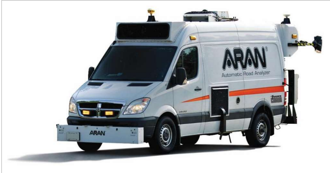
FIGURE 6 Mobile Van Used to Collect Data for Roadway Information Database.
