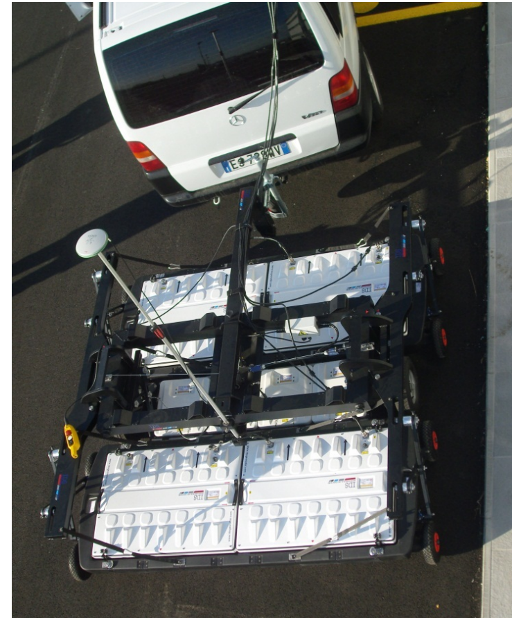
Stream EM System: complete configuration including 3 array of antennas
