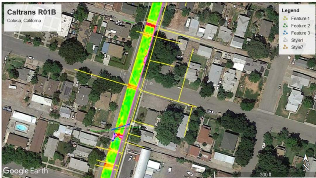
Figure 7. Screen capture. Draft 2D plan map (overlay on Google Earth Imagery) from TDEMI data collection – (known metallic utilities shown as thin yellow lines for comparison). Courtesy of Caltrans.
