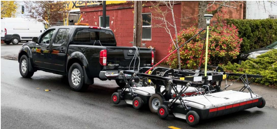
Figure 4. Photo of MCGPR towed array during R01B project work. Courtesy of Cardno.
