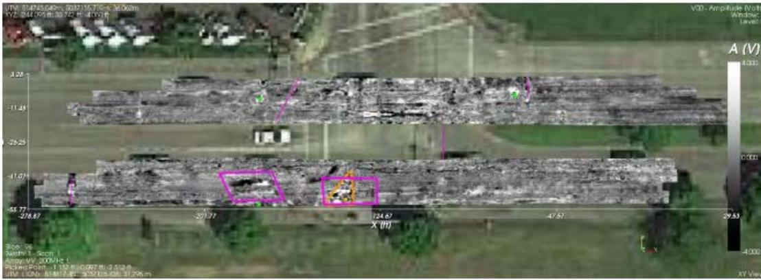
Figure 8. Screen capture. 2D image from 3D volumetric data taken with MCGPR array at 2.512 feet below road surface – (vaults and known utilities identified in purple). Courtesy of Cardno.
