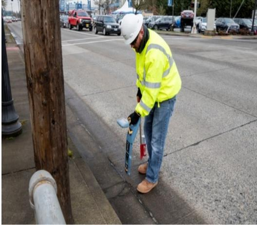
Figure 1. Example EMI SUE instrumentation (RD8100) – photo courtesy of Cardno
