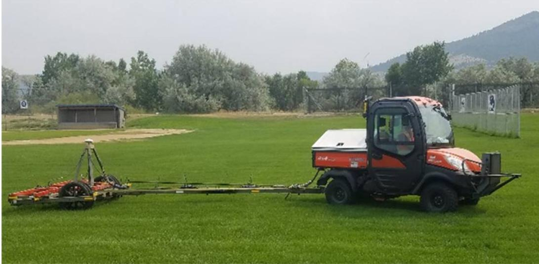
*Figure 5. Photo of TDEMI towed array during R01B project work. Note this is a diesel-powered tow vehicle. Courtesy of Utility Mapping Service, Inc.*
