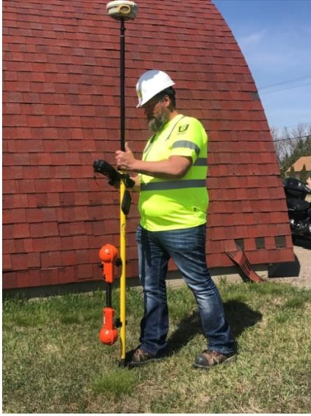
Figure 3. Example MAG SUE instrumentation (Vivax-Metrotech Spar 300 with GPS) – photo courtesy of Utility Mapping Services, Inc.
