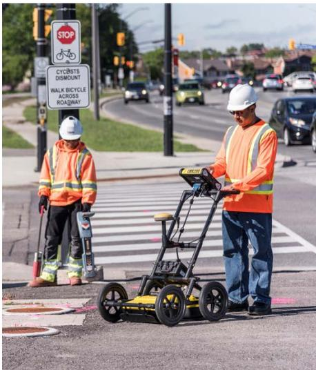
Figure 2. Example GPR SUE instrumentation (Sensors and Software LMX200™ GPR) – photo courtesy of Sensors and Software.
