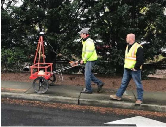
*Figure 14 Instrument technician focused on the data logger and GPS track mapper. Photo courtesy P. Sirles*
