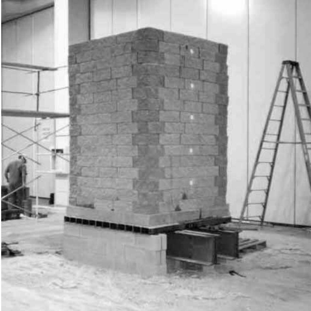
Figure 88. Photo. Vegas Mini-Pier Experiment reaction base.
