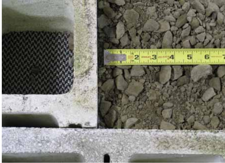
Figure 5. Photo. Sample of VDOT 21-A gravel.
