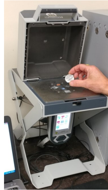
Figure 4, Pressed powder pellet as it comes out of the hydraulic press holder (left image) and placing of the pellet in the XRF test stand for laboratory analysis (photos courtesy of Maine DOT)
