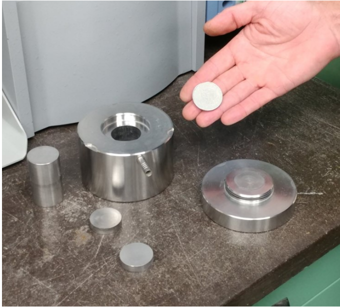
Figure 4, Pressed powder pellet as it comes out of the hydraulic press holder (left image) and placing of the pellet in the XRF test stand for laboratory analysis (photos courtesy of Maine DOT)
