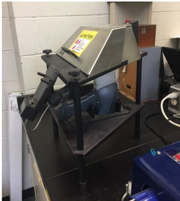
Figure 5, Example of XRF test stand, with a protective shield to isolate X-rays. Samples are placed within the shield in contact with the XRF window.
