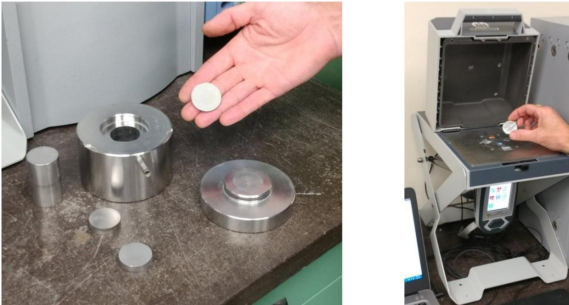
**Figure 4. Pressed powder pellet (left and placing of the pellet in the XRF test stand for laboratory analysis (photos courtesy of Maine DOT)**
