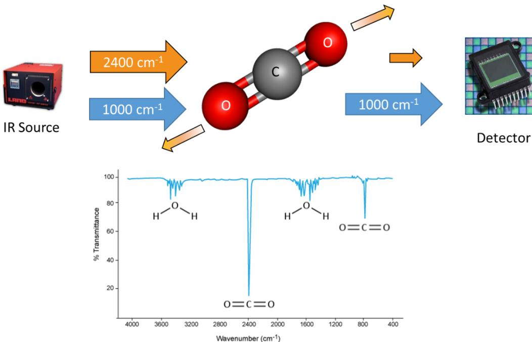
**Figure 9. Principle of molecular vibration upon IR irradiation of a  $\text{CO}_2$  molecule and corresponding spectrum.**
