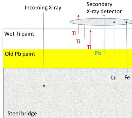
**Figure 7. Representation of the X-ray path as it is emitted from the XRF equipment, interacts and with the matrix and then re-emitted from different elements towards the detector.**
