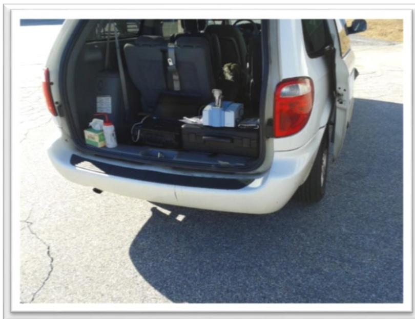
**Figure 12. Field Use of a benchtop ATR FTIR Spectrometer**
