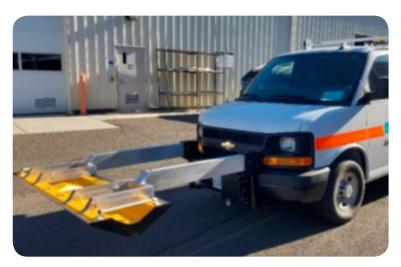
A 3D-GPR System. This is a Caltrans unit which shows the most current permanent mounted antenna design. Photo courtesy of Caltrans.
