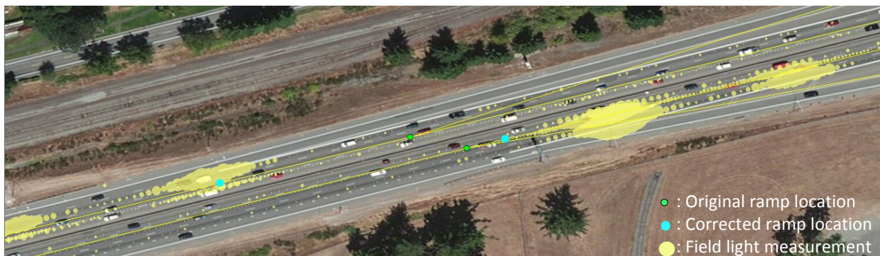
Figure 3. Corrected Ramp Locations on I-5.
