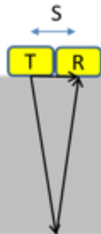
Ground coupled GPR
