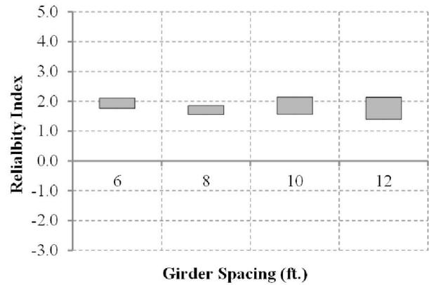
Figure 5. Reliability Indices of Various Bridge Decks Over A 1 Year Return Period (ADTT=5000), Positive Moment Region, Class 1 Exposure
