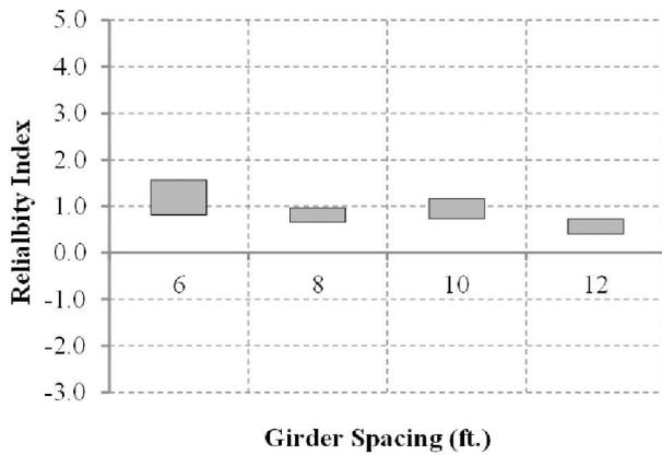
Figure 8. Reliability Indices Of Various Bridge Decks Over A 1 Year Return Period (ADTT=5000), Negative Moment Region, Class 2 Exposure
