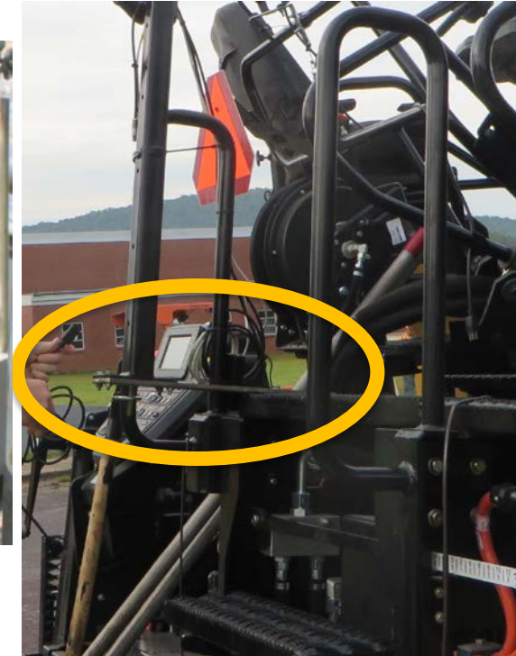
Mounted to a Steel Plate Attached to Work Platform
