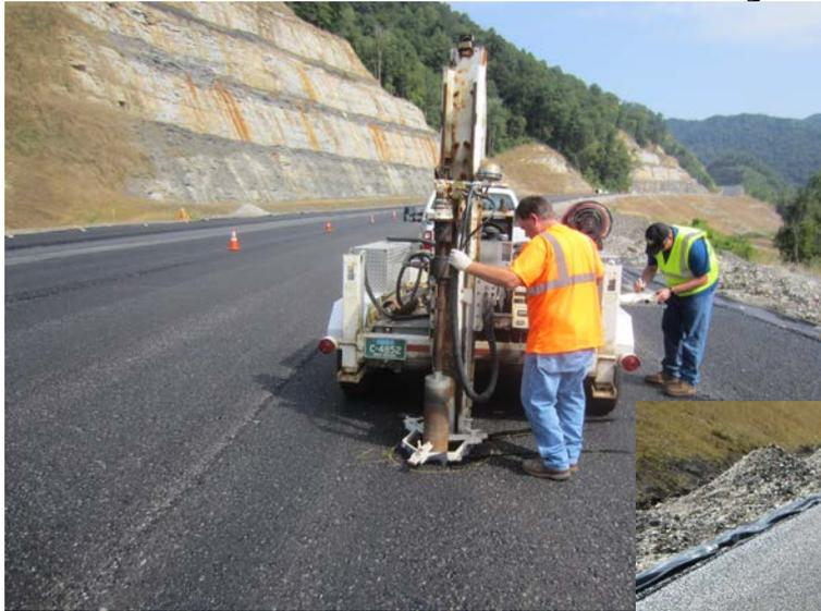
Cores, Nuclear & non-nuclear density gauge used to measure mat density and superimposed on temperature profiles.
