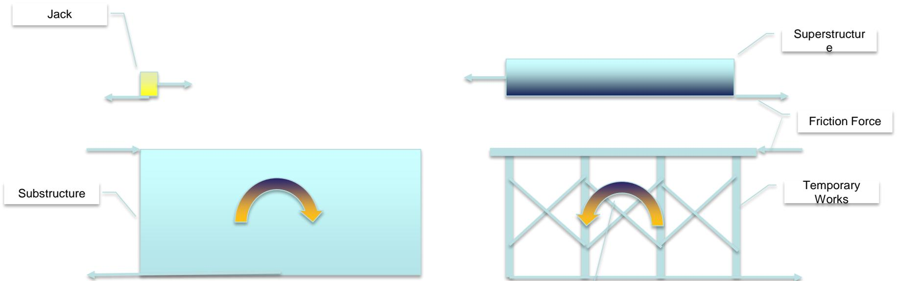
Unattached temporary works results in an overturning moment at temporary bent
