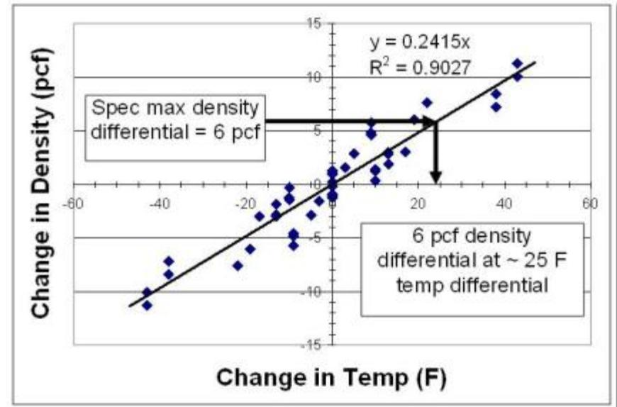
Temperature profile criteria based on desired density uniformity.
