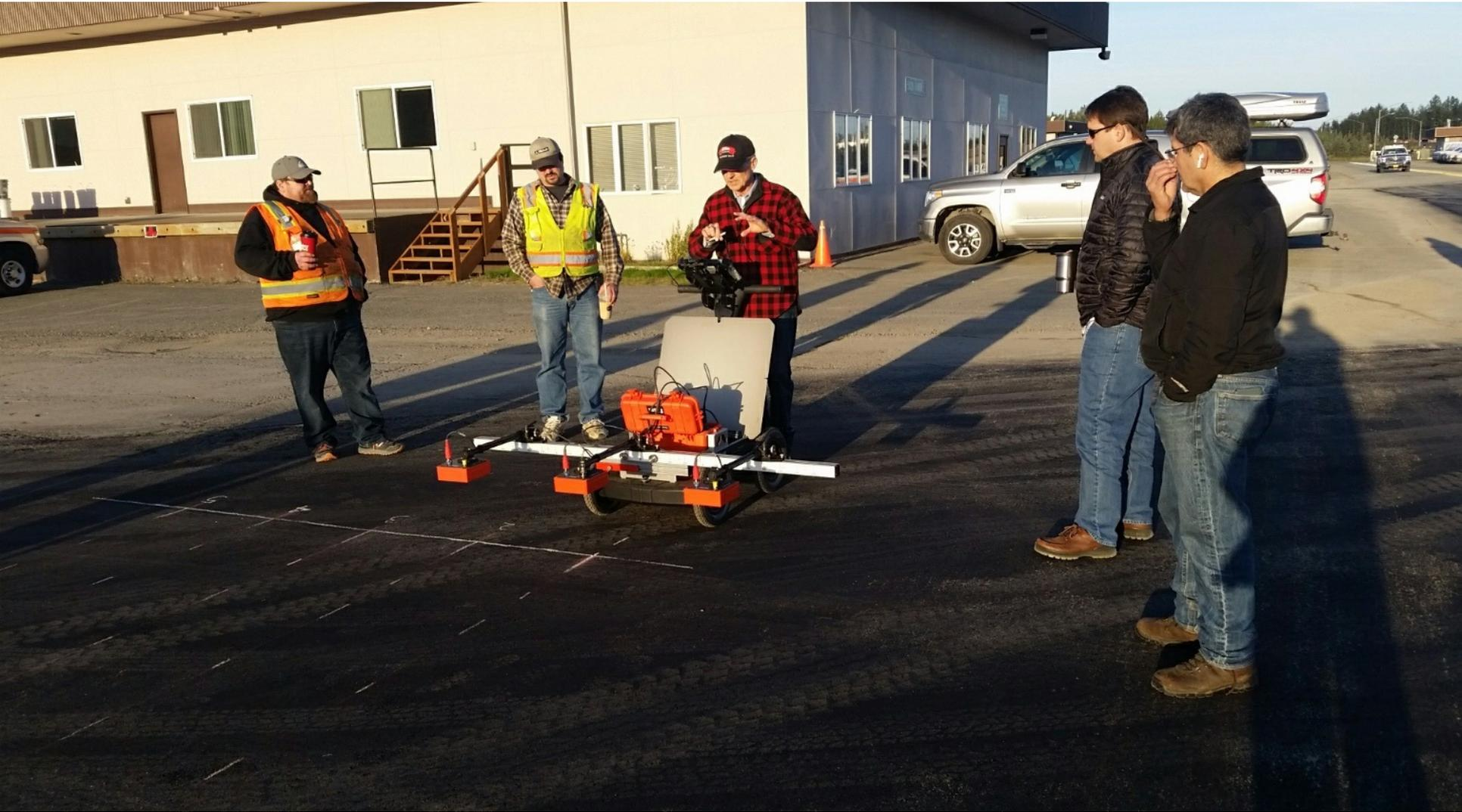
Position PaveScan with center antenna right at the marked starting point of Line 1.
