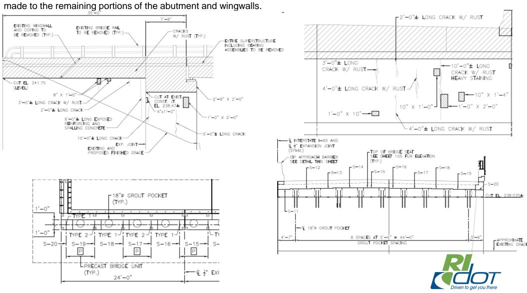
**Abutment Repairs and Precast Caps**
