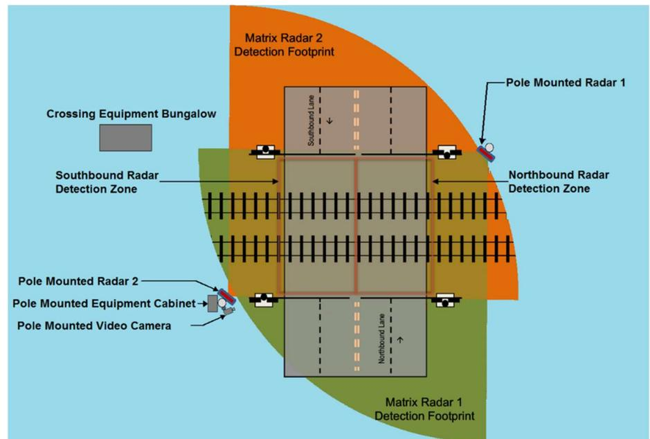
**Vehicle Detection System from Island Radar**
