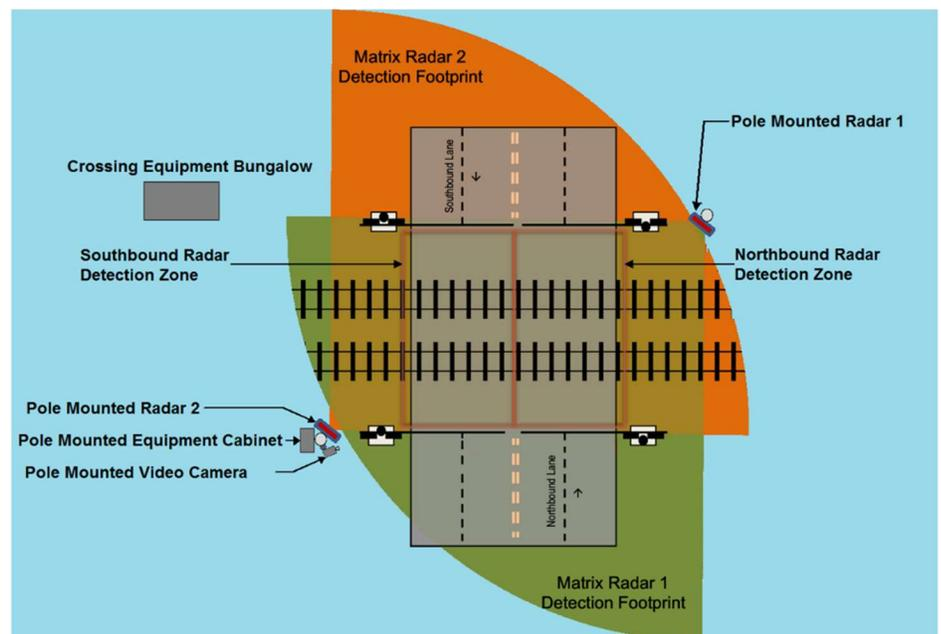
**Vehicle Detection System from Island Radar**
