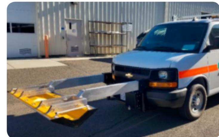
A 3D-GPR System. This is a Caltrans unit which shows the most current permanent mounted antenna design. Photo courtesy of Caltrans.
