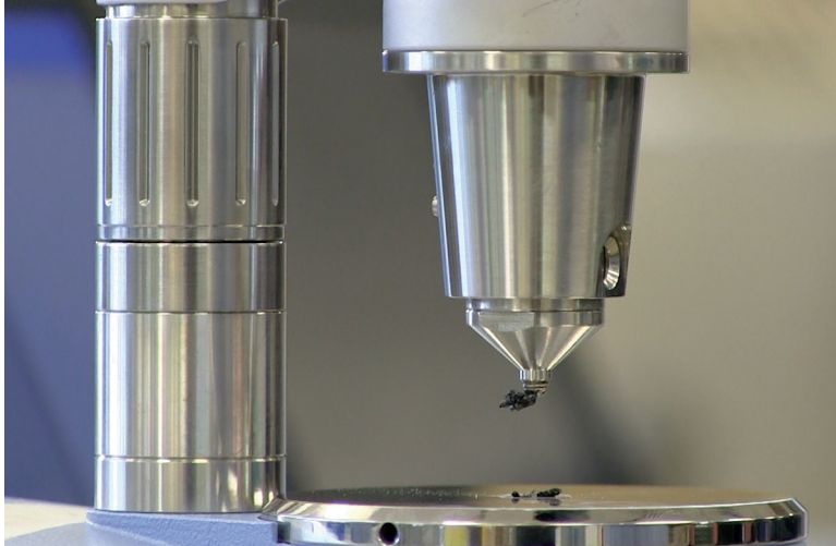
FTIR spectrometer testing an asphalt grain.
