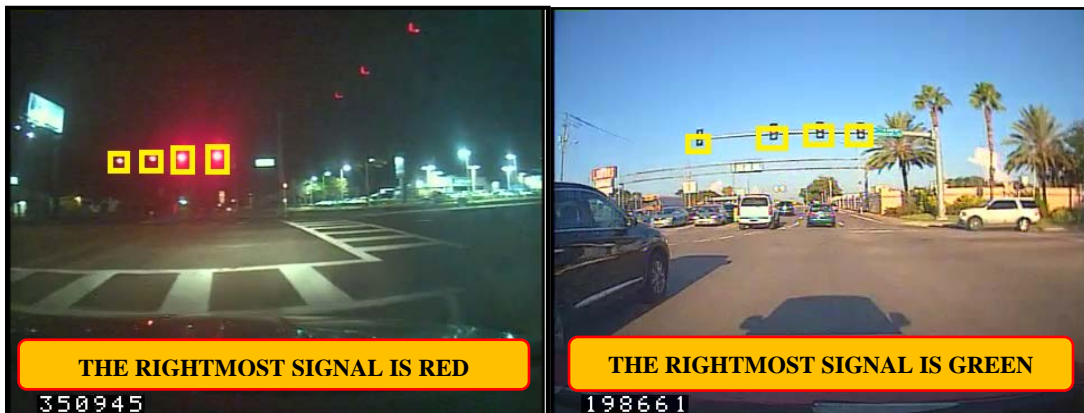
Figure 2. Example of traffic signal detection using NDS Automatic Video Processing Tool
