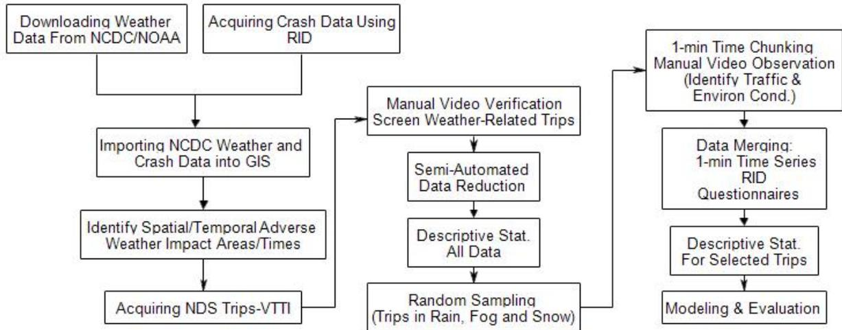
**Figure 2 Conceptual Overview of Phase 2 Data Acquisition and Preparation**
