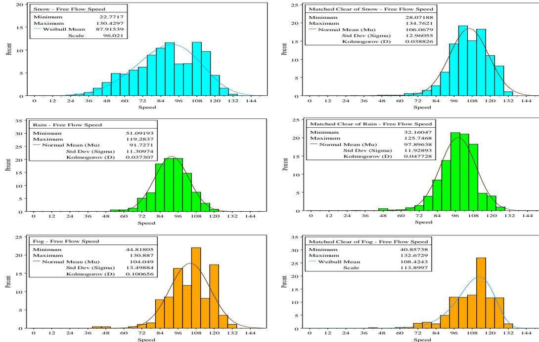
Figure 3 Observed and Fitted Distributions for Speeds during Adverse and Clear Weather under Free-Flow Traffic
