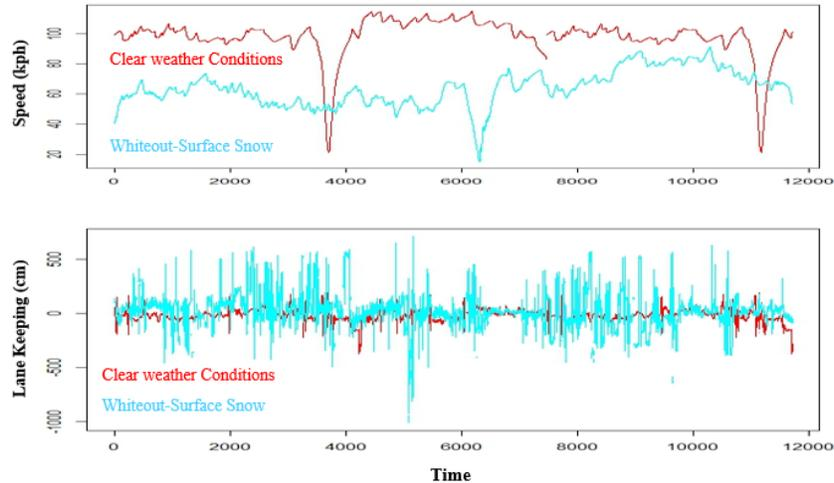
**Figure 6 Time-Series Speed and Lane keeping Performance in Clear and Whiteout- Snowy Surface Condition**
