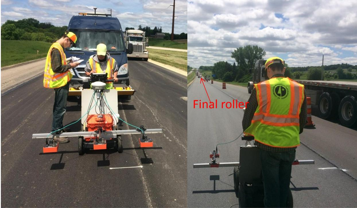
**Figure 1. Equipment and Data Collection [A] prior to a 500 ft pass, and [B] during data collection moving behind the final roller compactor.**
