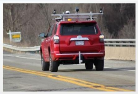
The technology used was the Deck Top Scanning System (DTSS) which is a mobile platform that can be loaded/mounted onto a vehicle. It consists of an infrared thermography (IR) camera, two line-scanning cameras, a GPS unit, and a speedometer unit that, combined, locate surface and sub-surface defects in bridge decks or roadways.
