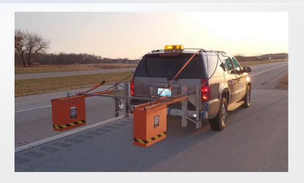
The technology used was a dual 2 GHz horn antenna system manufactured by GSSI, Inc. of Nashua, NH, The survey vehicle was equipped with an electronic distance-measuring instrument (DMI) mounted to the rear wheel of the survey van, providing continuous distance data as the GPR data was collected. The data collection and recording was controlled by the SIR-30 GPR system operated from within the survey vehicle.
