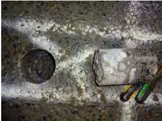
Core From BR08588B Showing Overlay (right), and Parent Material (left)
