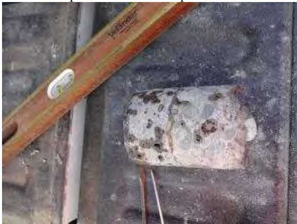
BR09259: Core Showing Overlay (left), Parent Material with Large River Rock (Right)
