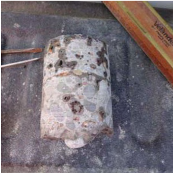
Core Sample Demonstrating Concrete Quality Comparison Between Original Construction and Rigid Overlay
