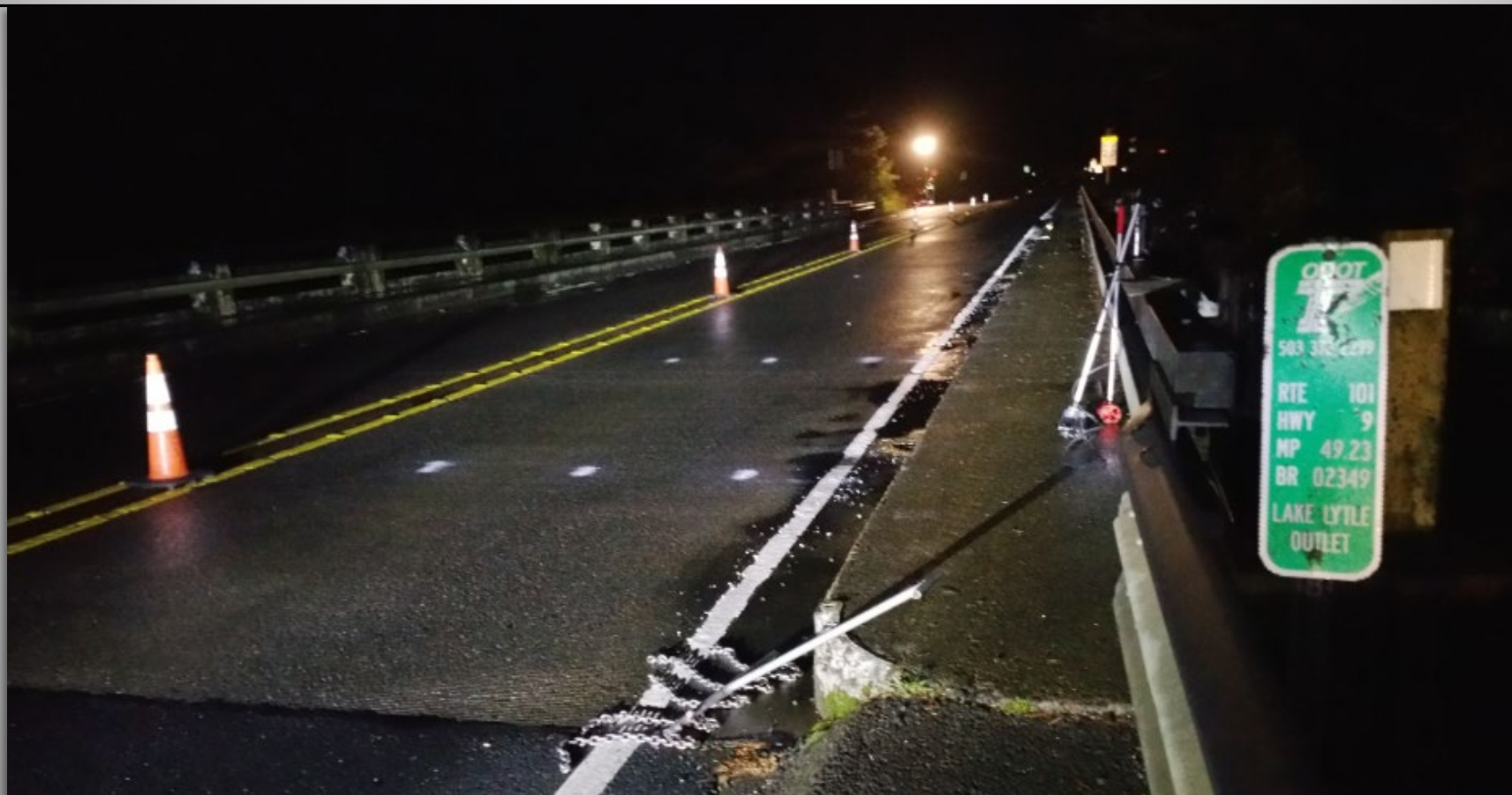
Image 5: chain drag and impact echo on Br 023948
