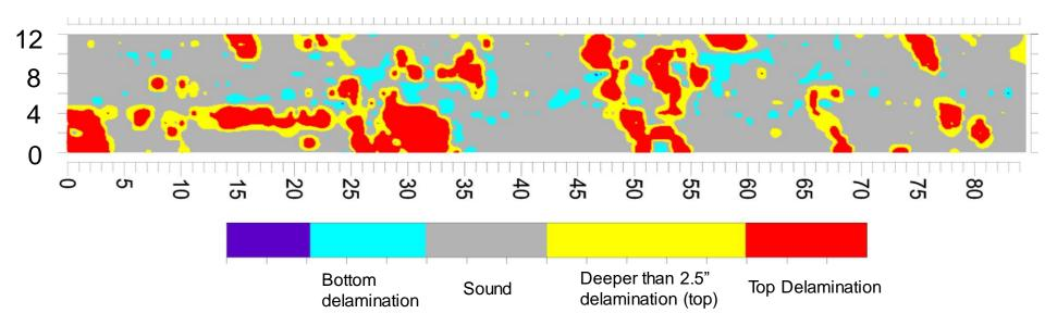
Areas with Probable Top Delaminations = 14% Areas with Probable Incipient (Deeper)Top Delaminations = 13% Areas with Probable Bottom Delaminations (or Thin Section) = 5.7%
