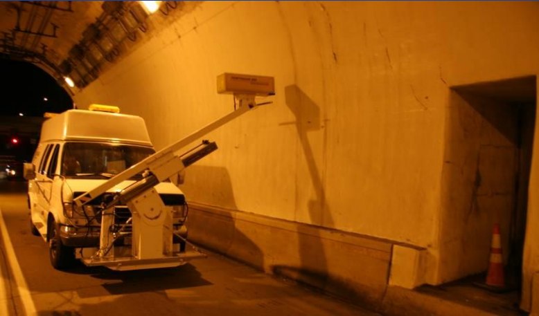
Penetradar GPR of PennDOT Tunnel
