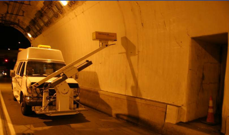
Penetradar GPR of PennDOT Tunnel
