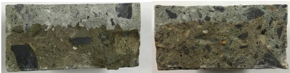
Figure 7: Split specimens with silver nitrate solution
