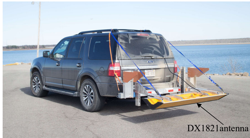
Figure 1 – 3D GPR survey vehicle setup
