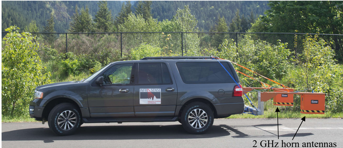
Figure 4 – Conventional GPR horn antenna system for bridge deck surveys
