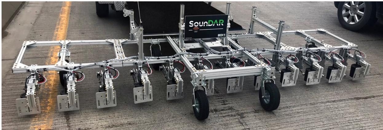
Figure 10 – Deck Acoustic Response (SounDAR) System
