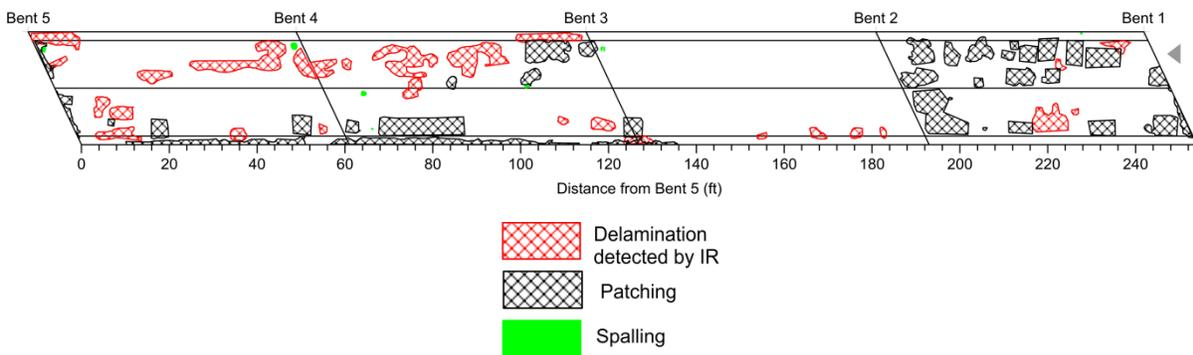
Figure 9 – Sample Finalized Plan Area Map Showing IR Delaminations, Visual Patches, and Spalling
