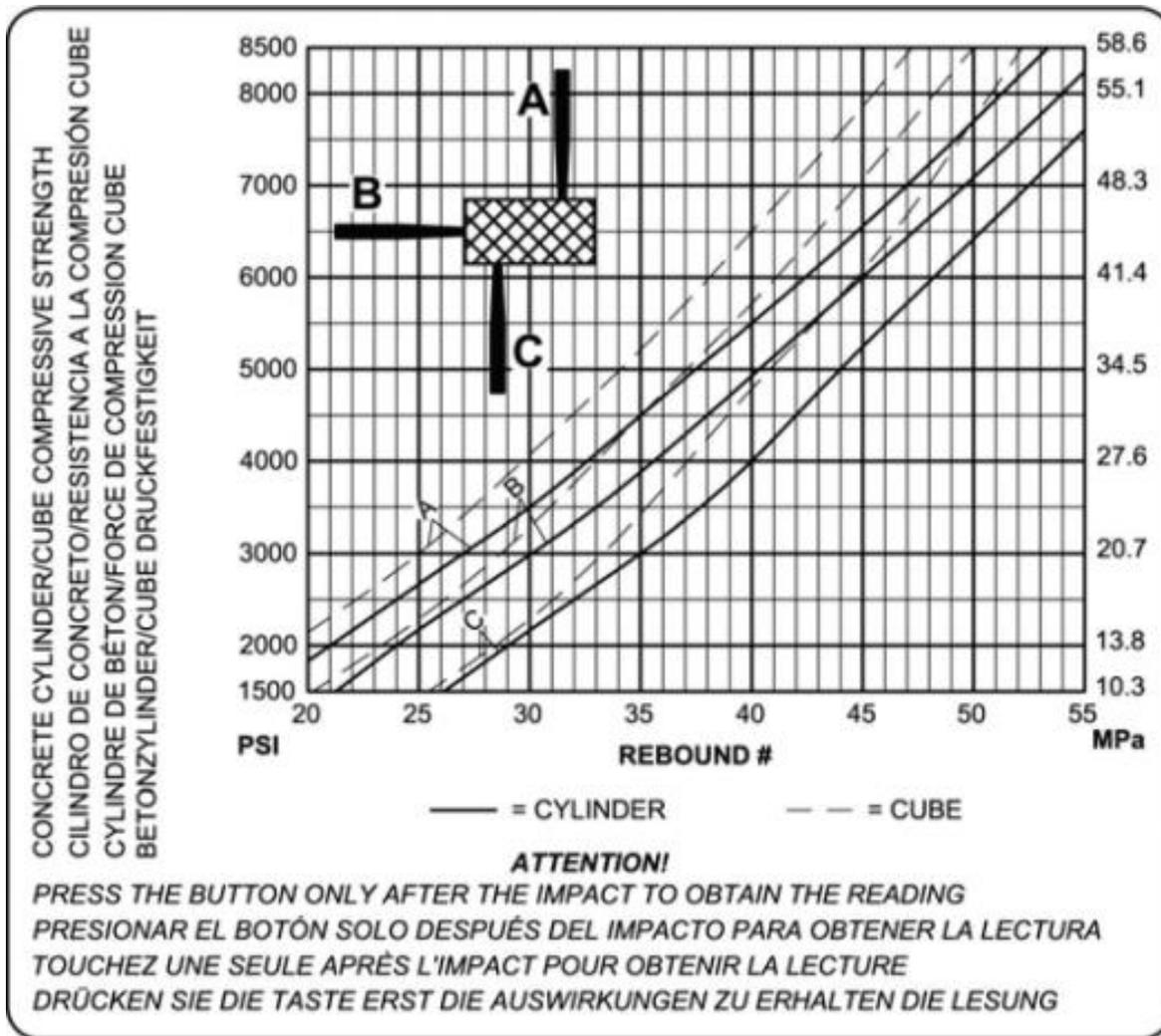
Figure 14 – Rebound Hammer Measurement Conversion Curves
