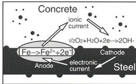
Figure 11 – Process of Corrosion in Structural Concrete.
