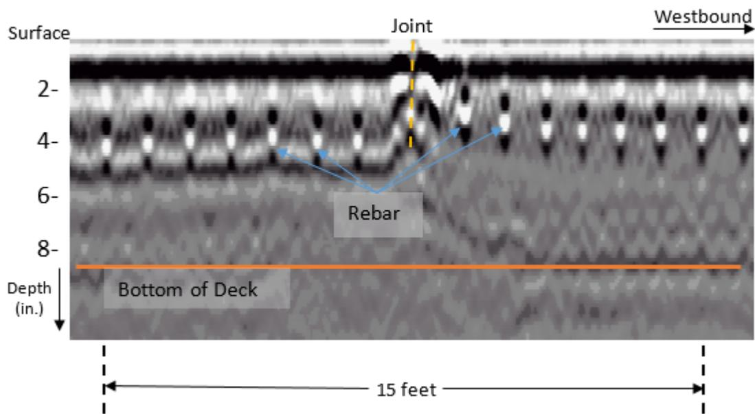
Figure 2 - Sample GPR Data Showing Consistent Rebar Reflections and Varying Depths
