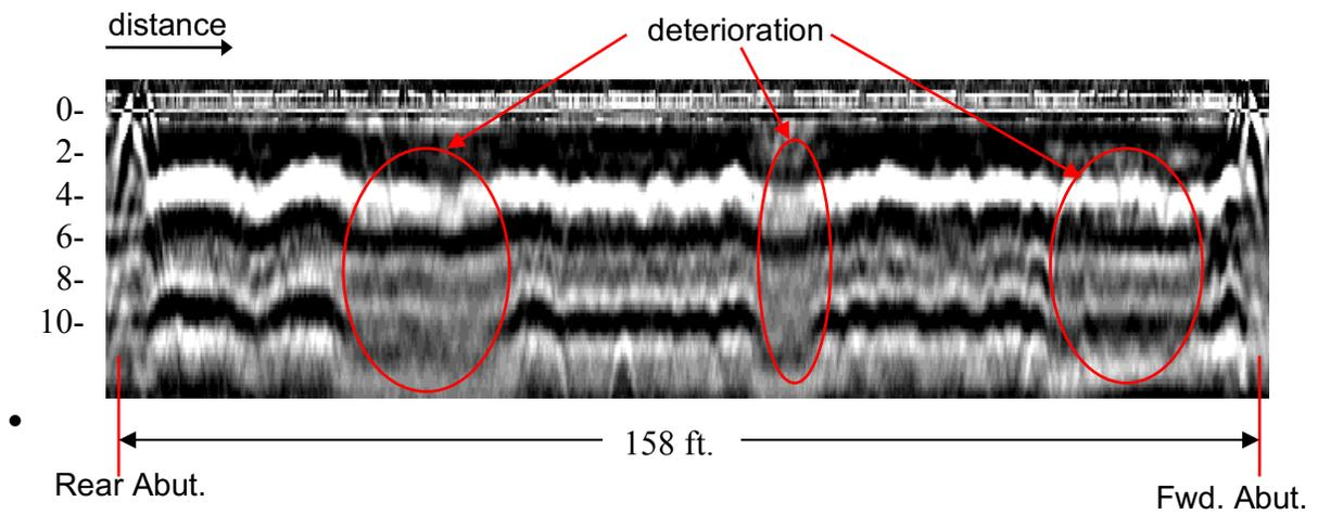
Figure 4 – Sample GPR Bridge Data with Probable Areas of Deterioration
