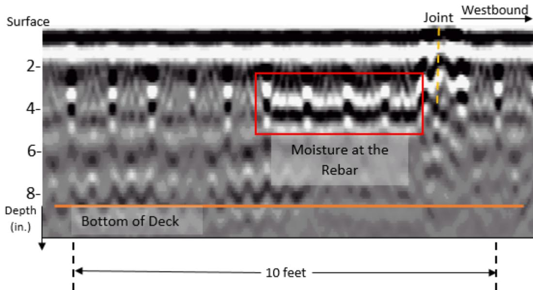
Figure 3 - Sample GPR Data Showing Evidence of Moisture at the Bottom of the Overlay
