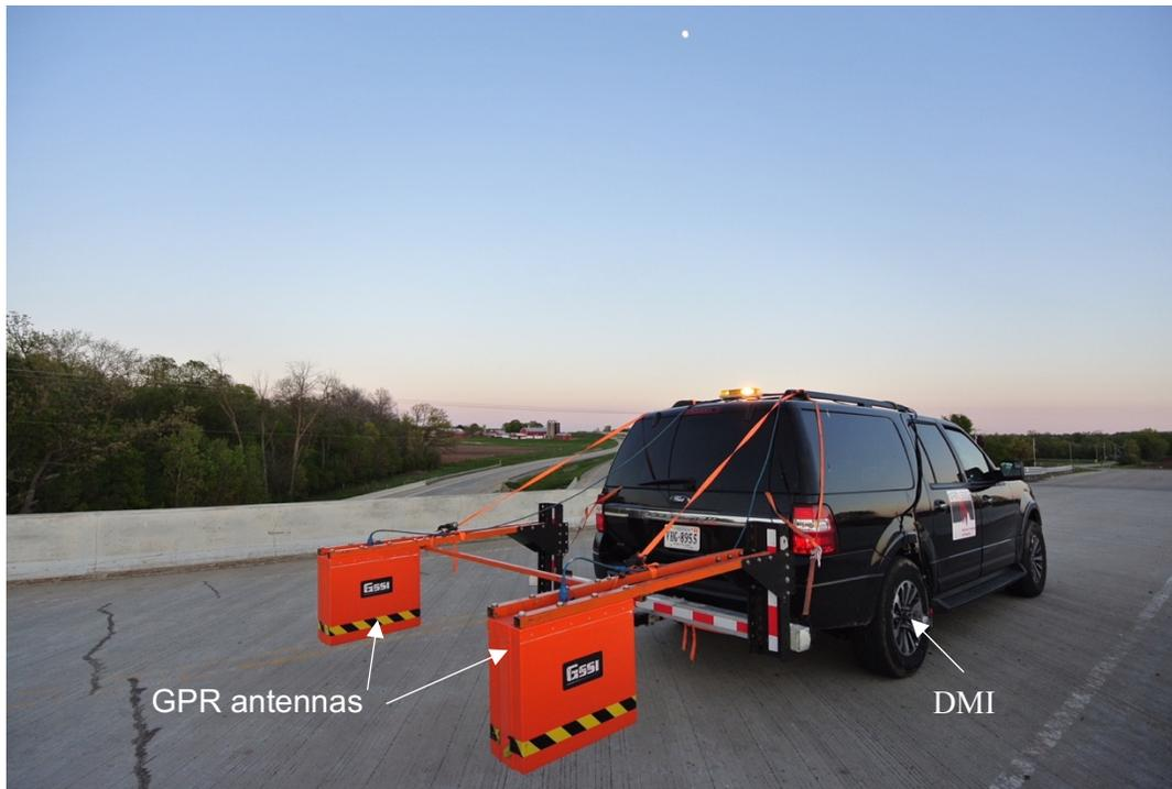
Figure 1 - GPR Survey Equipment
