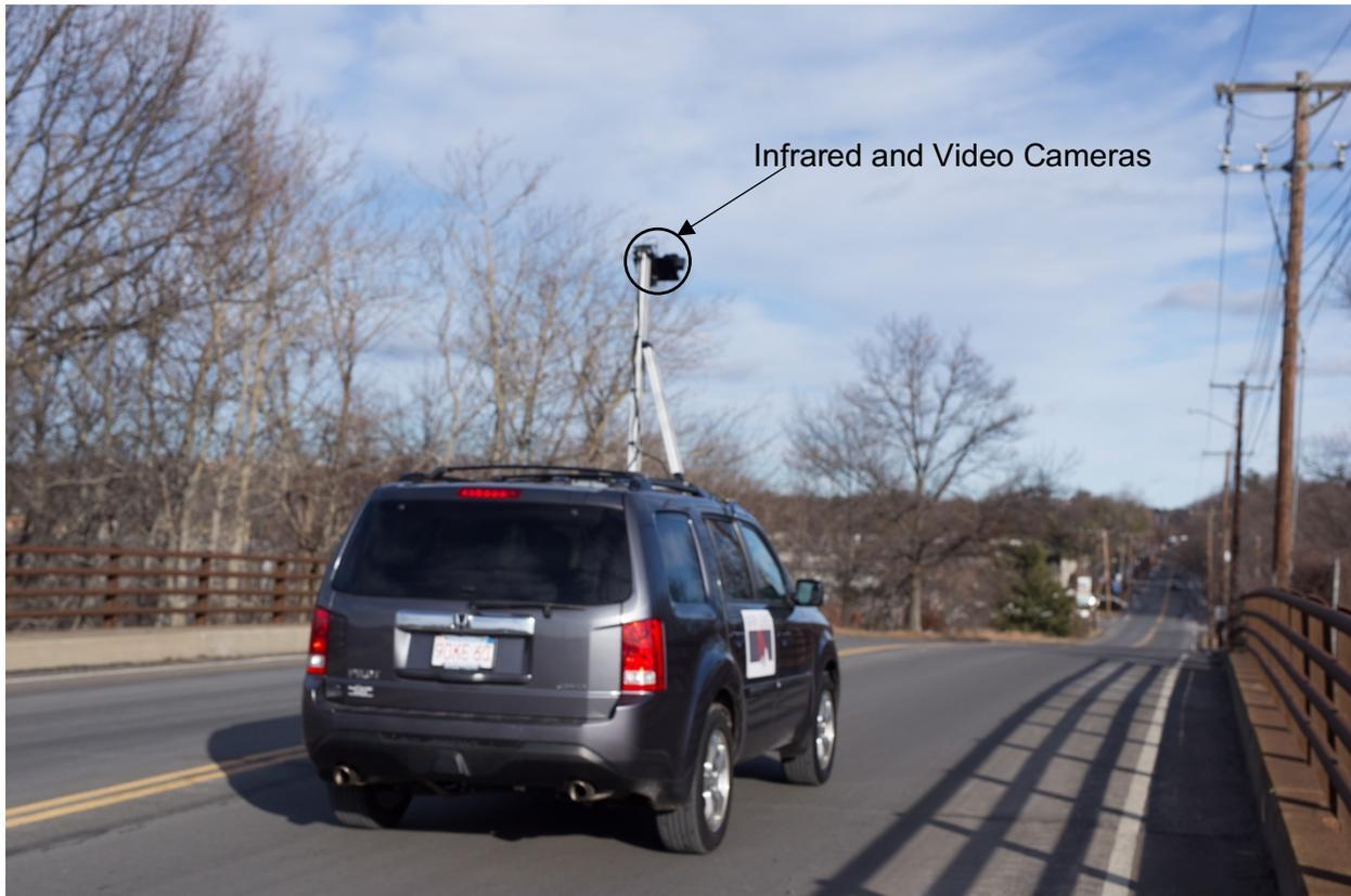
*Figure 6 - Infrared and Video Survey Equipment*
