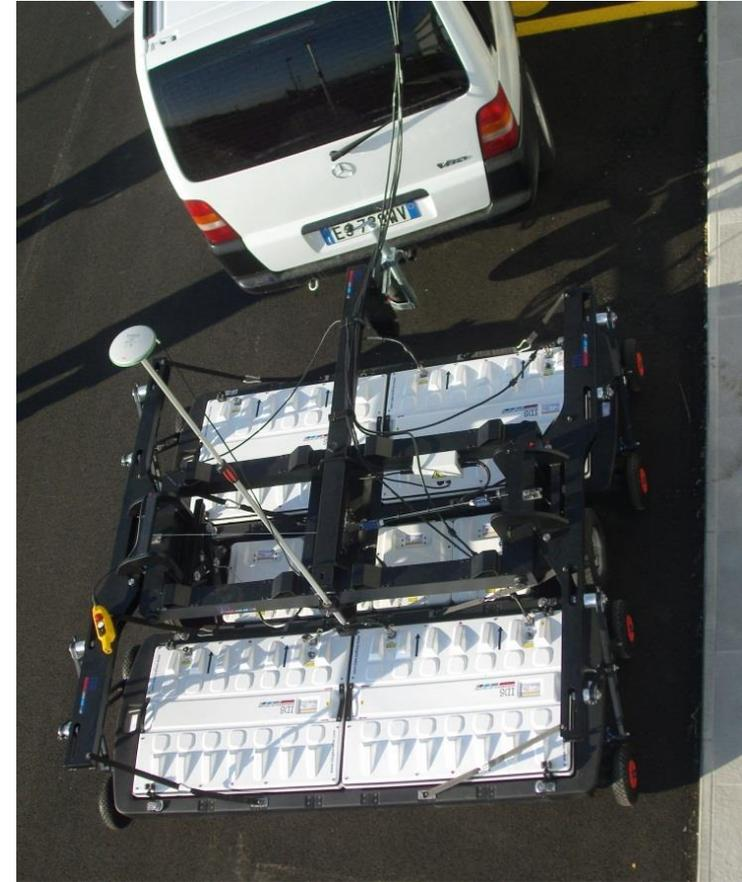
**Stream EM System: complete configuration including 3 array of antennas**
