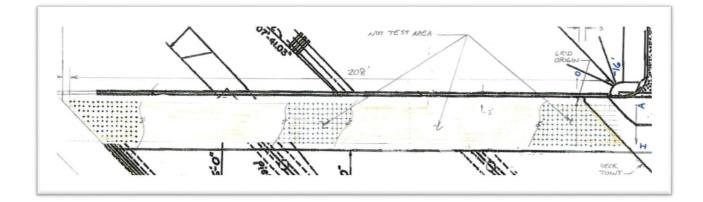
Objective was to obtain top (and bottom) delamination location and quantities at the test site for the various rapid IE methods. This was a project-level experiment (versus a system-wide evaluation).
