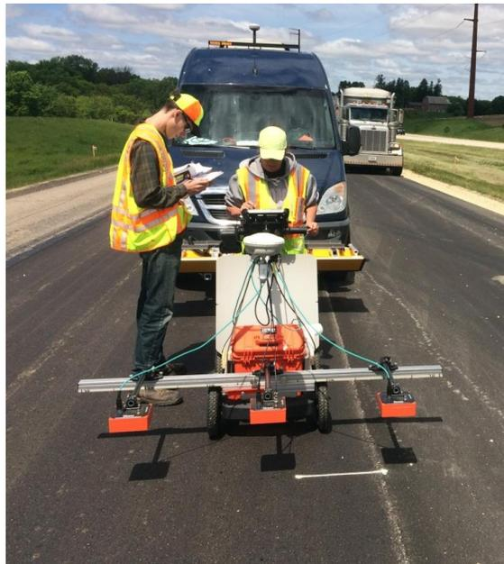
**Figure 2. Three-sensor Rolling Density Meter Configuration via Extended Cart**
