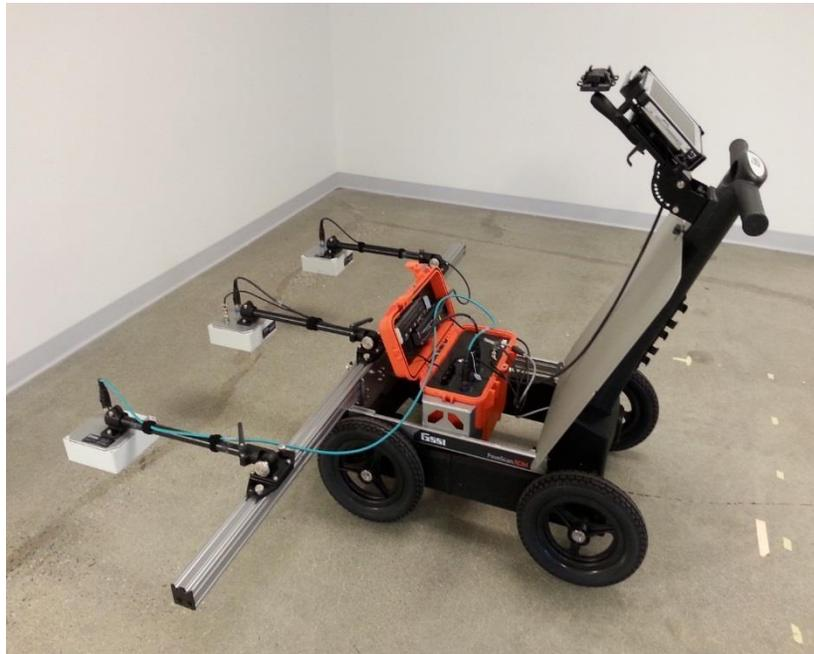
**Figure 1. Rolling Density Meter**
