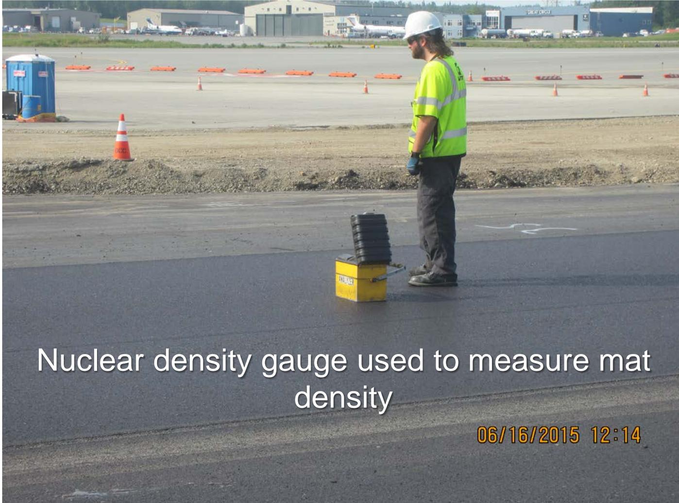
Nuclear density gauge used to measure mat density
