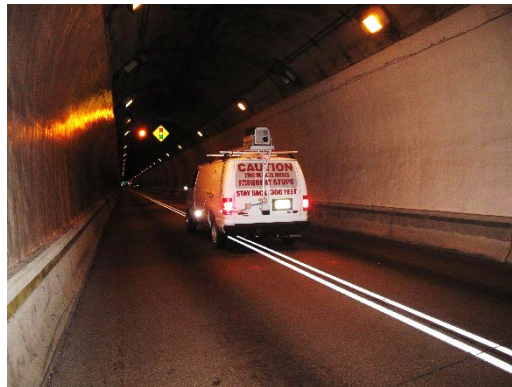
Photo 12: SPACETEC scanning in Liberty Tunnel
