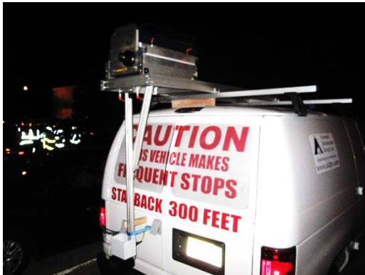
Photo 10: SPACETEC scanner on vehicle
