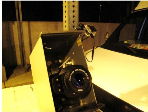
Photo 9: Close-up of IR and Video Camera
