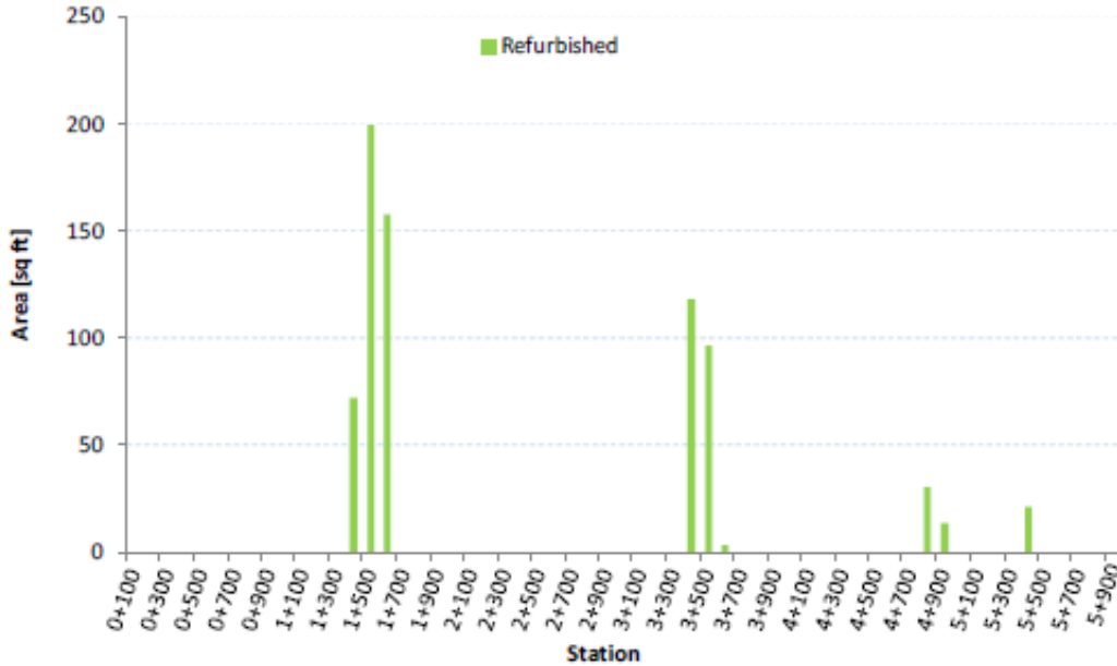
Figure 20: Distribution of Refurbished (Patched/Repair) Areas for Liberty Tunnel
