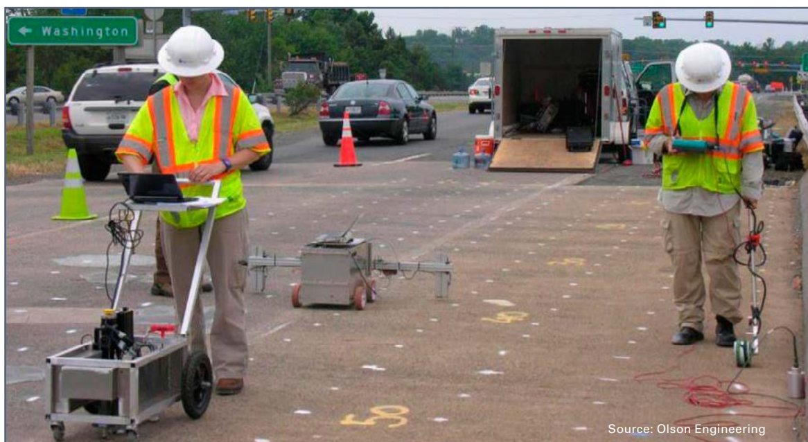
Nondestructive Testing for Concrete Bridge Decks in the field.
