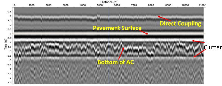
GPR reflection interference ("clutter") caused by vehicle proximity and mounting
