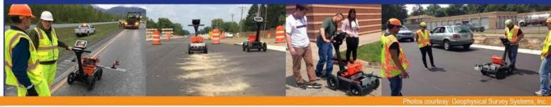
Asphalt Mixture Compaction Assessment Using Ground Penetrating Radar (GPR) Density Profiling Systems (DPS)
