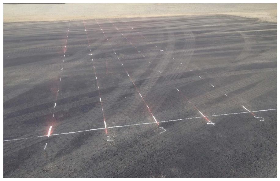
5 lines spaced 2' apart, each line 35' long. Note that only lines 2, 3, and 4 will be measured by all three antennas.
