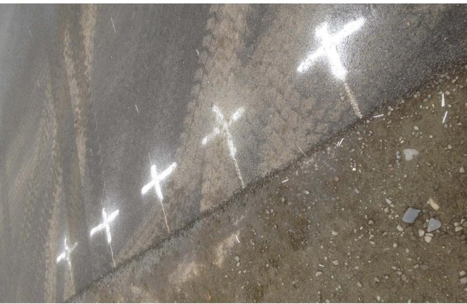
Place end marks one foot from paving edge to avoid inclusion of highly irregular readings at pavement edge.
