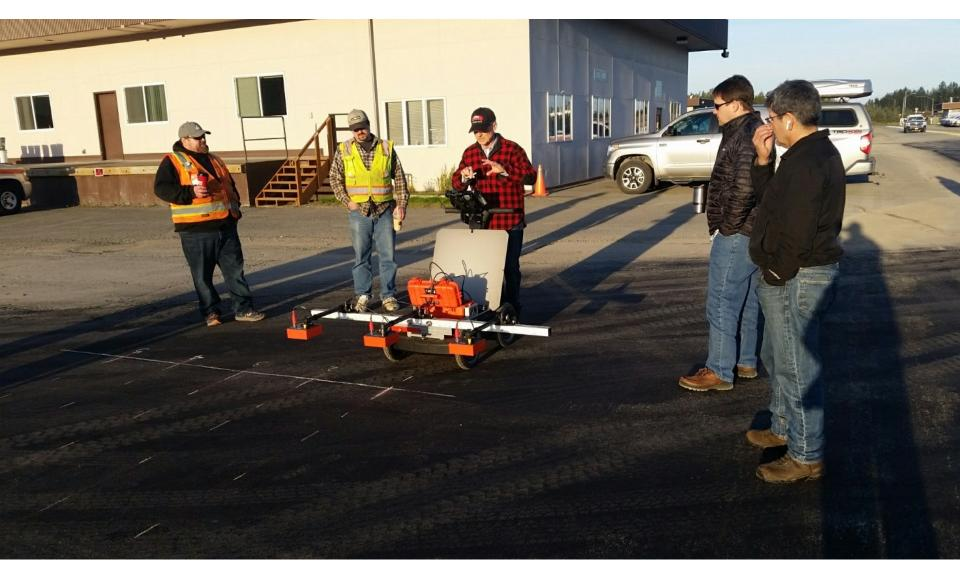
Position PaveScan with center antenna right at the marked starting point of Line 1.
