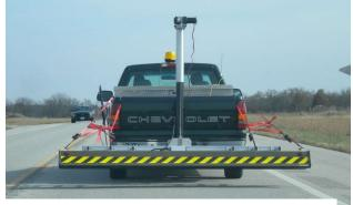
GPR Antenna Array (3-D Radar)
