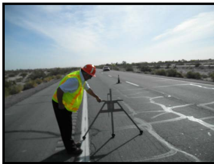
Figure 3.3: Rut Measurement on I-8
