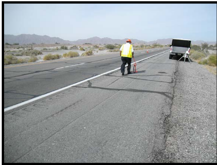
Figure 3.2: 100' Roadway Segment Identification for the Distress Evaluation Survey
