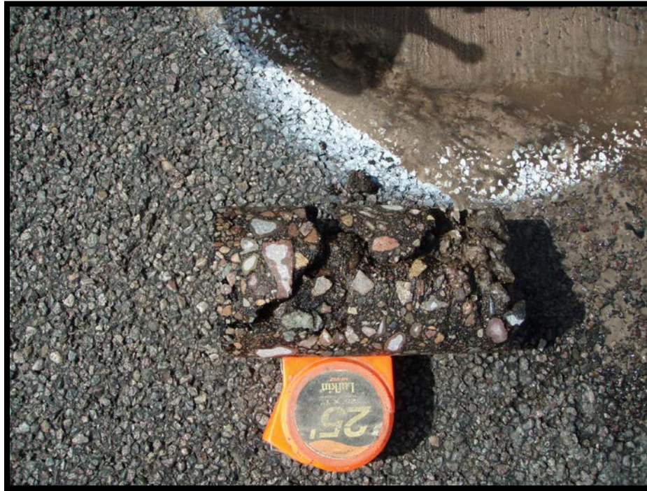
Figure 3.6: Pavement AC Layer Depth Measurement and Analysis
