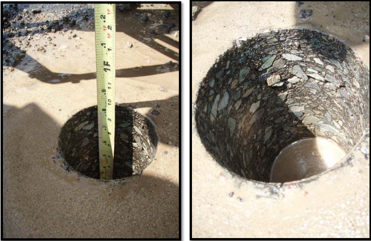
Figure 3.8: AC Core Depth Measurement on I-10 (WB)
