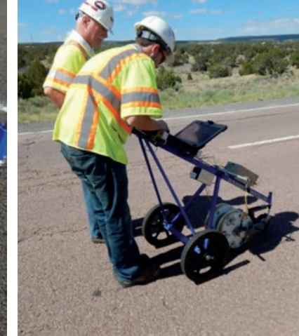
SASW/IE manual point testing (left) and automated testing (right). Photo on the right courtesy of Texas A&M Transportation Institute and the New Mexico Department of Transportation.
