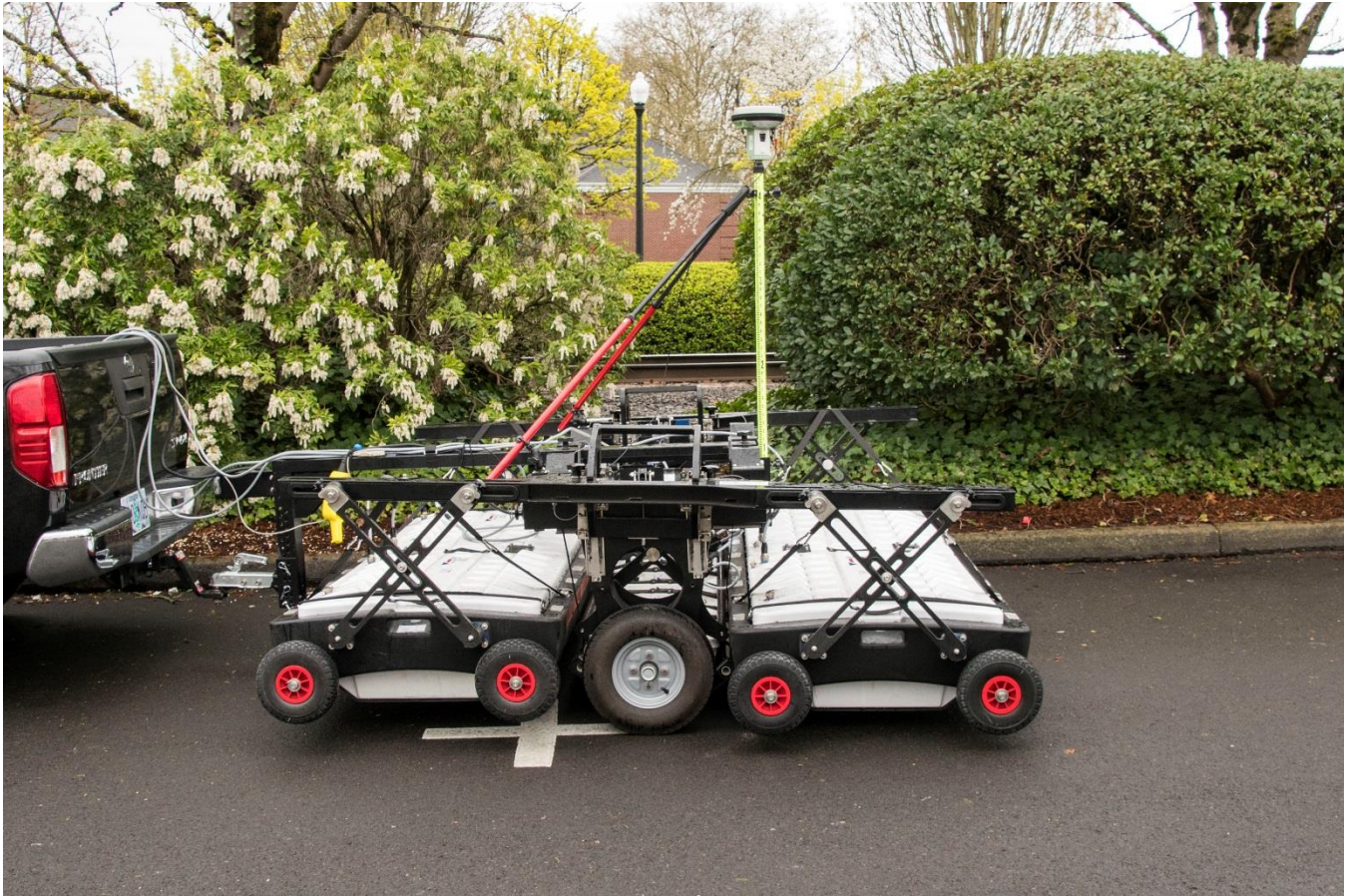
MCGPR instrumentation used during the SHRP2 R01B Utility Locating Technology program for the ODOT SR8 project. Shown here is the IDS GeoRadar Stream EM system, with RTK GPS mounted for centimeter positional accuracy of data. The Stream-EM consists of an array of 40 double-polarized GPR antennas, ranging in frequency from 200MHz to 600Mhz, where pipes, cables and buried utility anomalies are detected with high accuracy and can be individually distinguishable. (photo courtesy of Oregon DOT).
