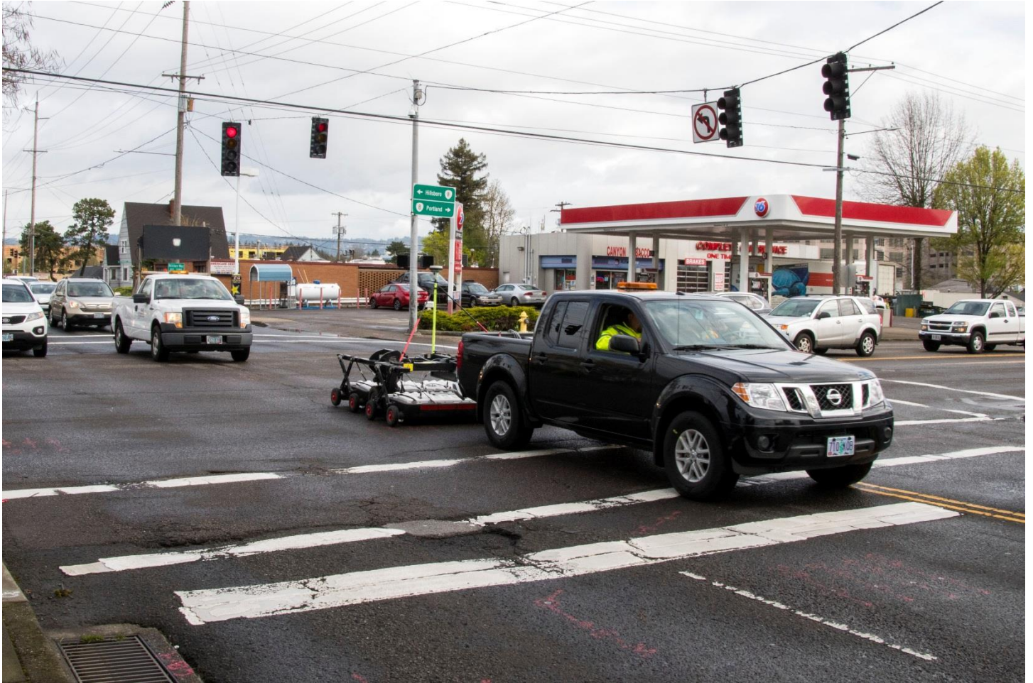
MCGPR data being acquired at the intersection of Oregon SR8 and Hocken Avenue during mid-day, utilizing a IDS Stream-EM system with RTK GPS. The vehicle can travel between 5 and 10 mph, with a chase/arrow vehicle to route traffic around the vehicle and MCGPR trailer system containing 40 GPR antennas (photo courtesy of Oregon DOT).
