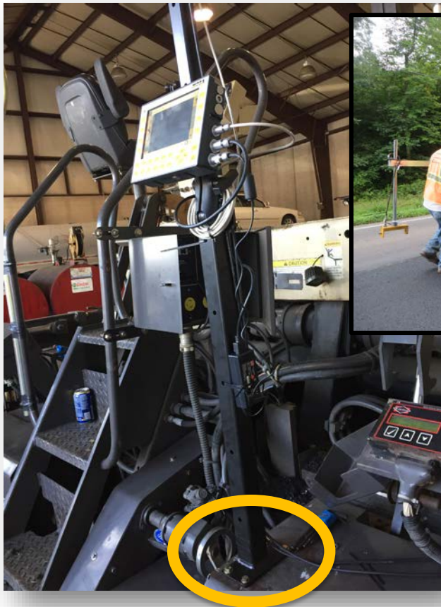
Mounted Directly to Screed
