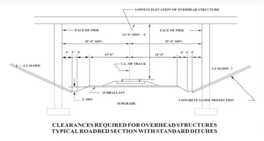
NOTE: FOR MULTIPLE TRACKS, STANDARD TRACK CENTERS IS 15\*0". AN ADDITIONAL 8\*-0" WIDE ACCESS ROAD MAY BE REQUIRED TO PROVIDE 33\*-0" MINIMUM DISTANCE FROM CENTERLINE OF TRACK TO FACE OF PIER.
