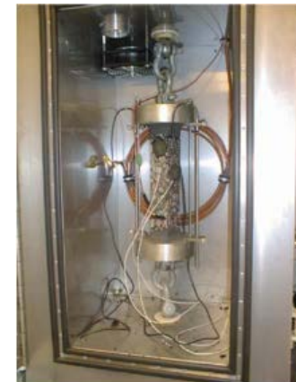
Thermal Stress Restraint Specimen Test Chamber
